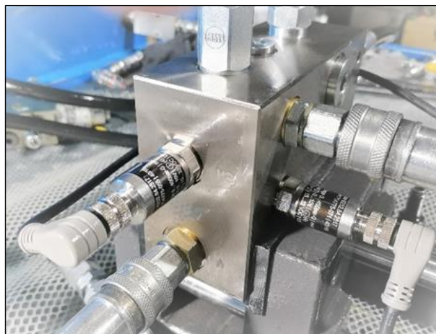
Customized manifold testing 定制阀组测试
